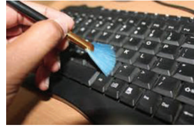
Figure 3.21: Cleaning keyboard with soft brush
